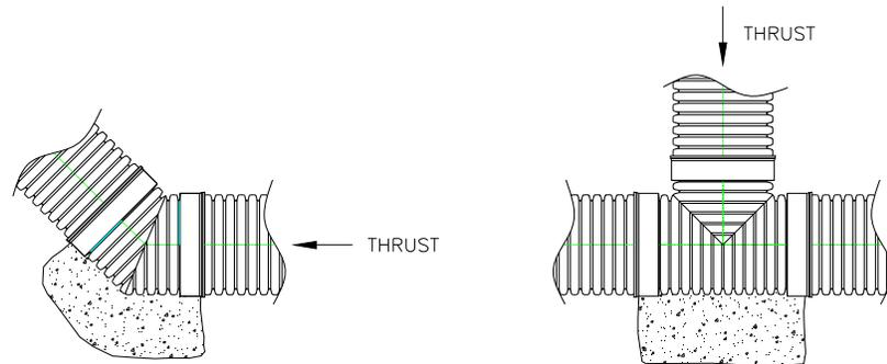
Precast concrete blocks may also be used, but should not be placed directly against the pipe to avoid point loads on the fitting. Backfill should be placed between the face of the precast block and the fitting in order to provide uniform support of the fitting.
