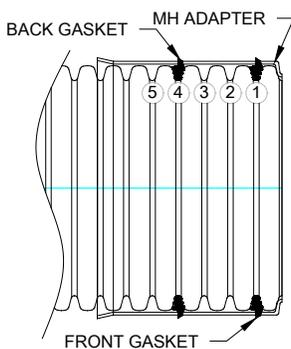
The gaskets are positioned in the 1<sup>st</sup> and 4<sup>th</sup> corrugation valleys.
