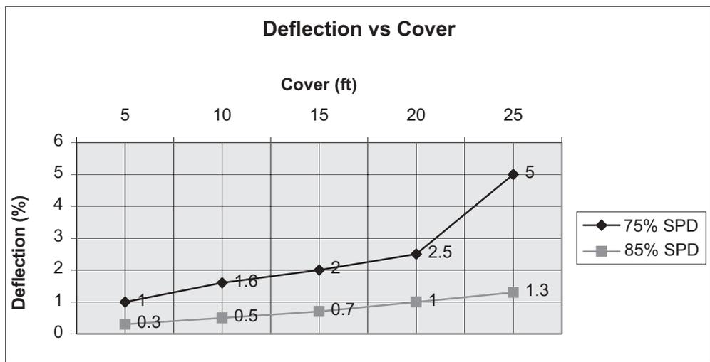
**Figure 1: Comparison of Deflection Values for 75% and 85% SPD Material**
